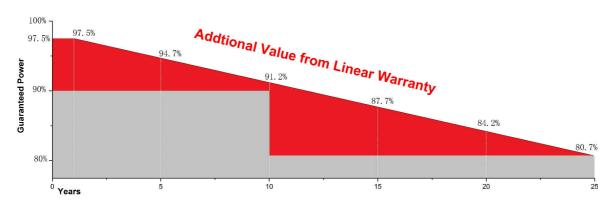
For Monocrystalline Products: less than 3.0% in the first year, thereafter less than 0.68% per year, ending with no less than 80.68% in the 25<sup>th</sup> year after the Warranty Start Date.
