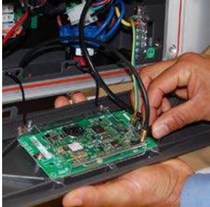
Disconnecting Display Module Connectors
