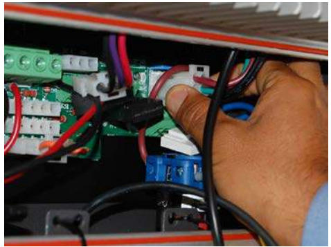
Connecting the Inverter Module
