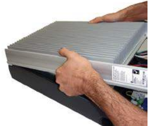
Removing the Inverter Module
