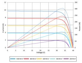
Excellent performance under weak light conditions: at an irradiation intensity of 200 W/m² (AM 1.5, 25 °C), **96.5**% efficiency (200 W/m²) is achieved.
