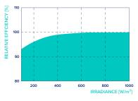
Typical module performance under low irradiance conditions in comparison to STC conditions (25 °C, 1000 W/m<sup>2</sup>).
