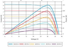
Excellent performance under weak light conditions: at an irradiation intensity of 200 W/m $^2$  (AM 1.5, 25 °C), 95.5% or higher of the STC efficiency (1000 W/m $^2$ ) is achieved
